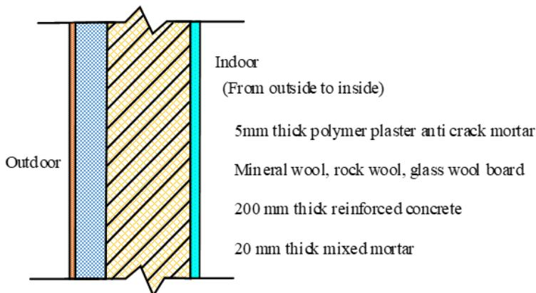
area is 10,376.14 m<sup>2</sup> and the building's height is 84.10 m. From indoor to outdoor, the construction levels of the building exterior wall are 5-mm-thick polymer plastering anti-cracking mortar, mineral wool, rock wool, glass wool board, 200 mm-thick reinforced concrete, and 20 mm-thick mixed mortar. The dry density of glass wool board is around 80-100.
