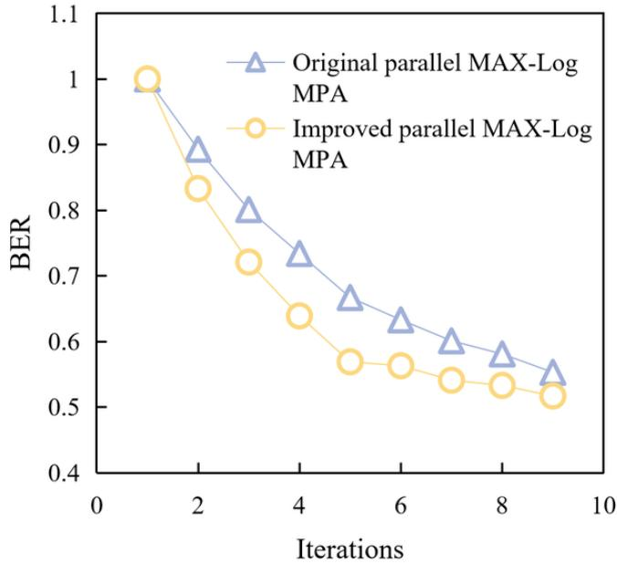
Figure 9. Comparison of serial MAX-log MPA BER before and after improvement
