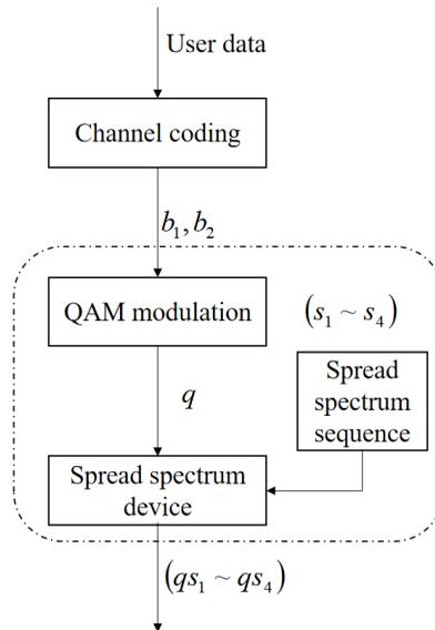
Figure 2. Schematic diagram of SCMA sender
