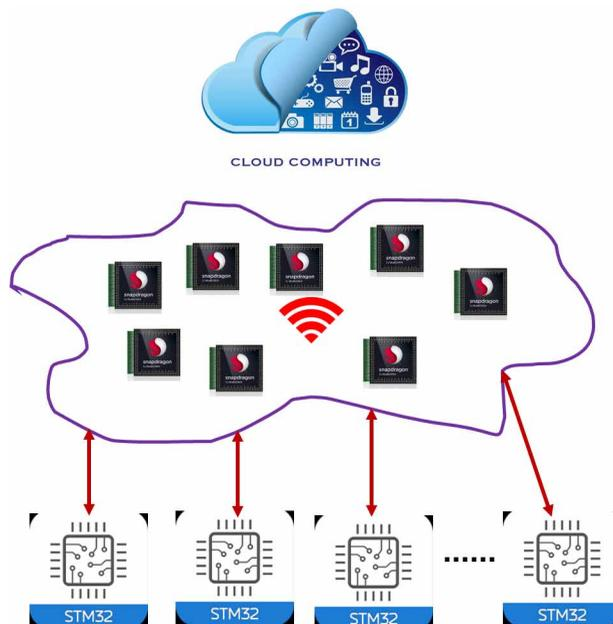
Figure 2. Hierarchical Model of Industrial Networks
