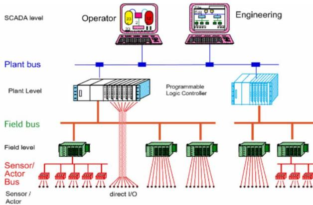
1. The device level, i.e., the network of sensors and actuators. The primary function at the device level is data acquisition and control.
