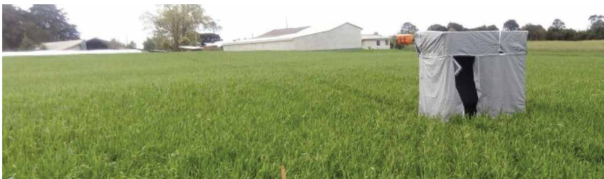
Figure 2. Blackout enclosure over the appliance at the field
