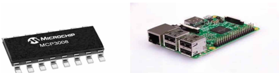
Figure 6. The MCP3008 microchip and Raspberry PI 3
