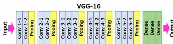
Figure 8. Schematic diagram of VGG 16 Model.
