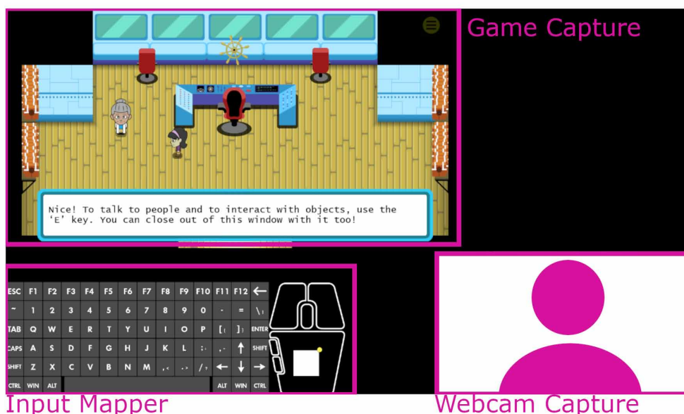
Figure 2. A screenshot of our instrument in OBS. Each data stream that is merged into the instrument is labeled. This is the view of the data collection instrument; however, the player only sees the ‘Game Data Stream’ window in full screen.
