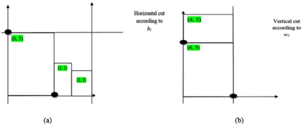
Figure 9. The last possible placement and the final cutting pattern. (a) The horizontal placement. (b) The final cutting pattern
