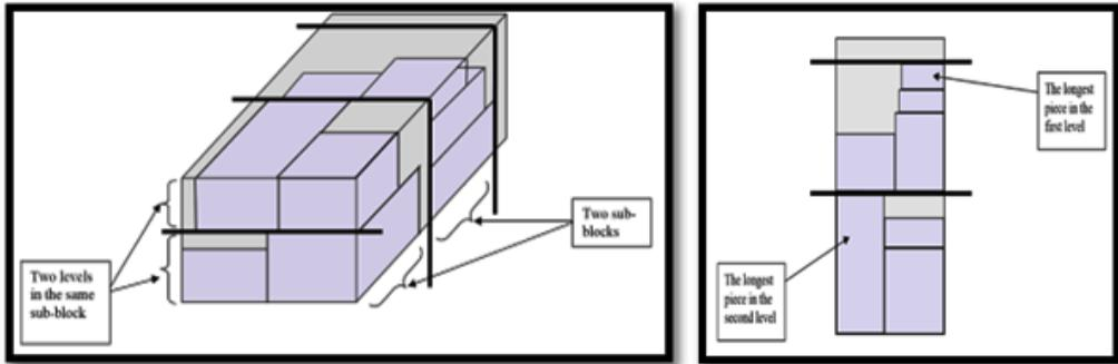
levels. The length of each sub-block corresponds to the longest piece (foam mattress) placed in its levels. The Fig.6. (b) shows a top view of the Fig.6.(a). It clarifies the composition of sub-blocks.
