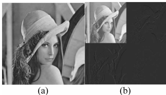
Figure 1. Wavelet Decomposition of Image Lenna: (a) Original Host Image Lenna, (b) Four Sub-Bands After the First-Level Wavelet Transform of Lenna
