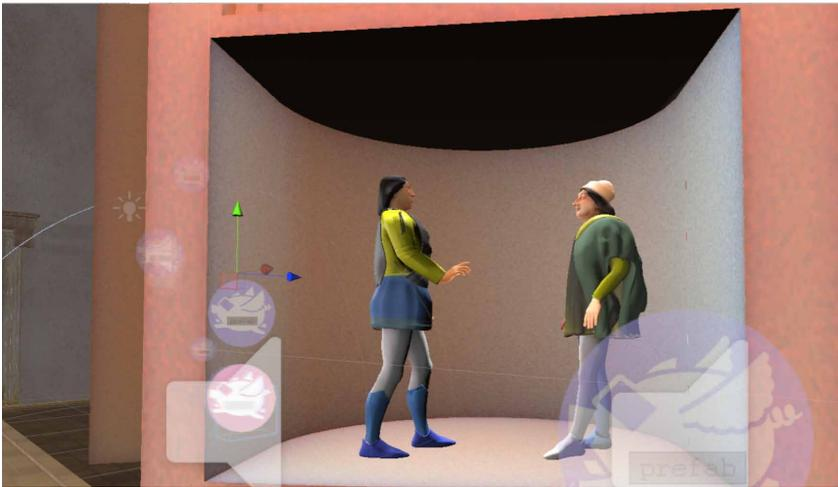
users can walk inside the physical/virtual enclosure, and when they trespass to its limits, the headset video signal stops and shows the surrounding area through video. In such a case, the play area can be expanded to provide more room for interaction and navigation via extended reality.
