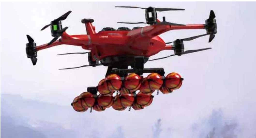
Figure 2. Drone equipped with extinguishing balls
