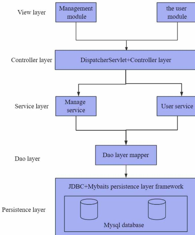
Figure 5. Functional structure design of the system
