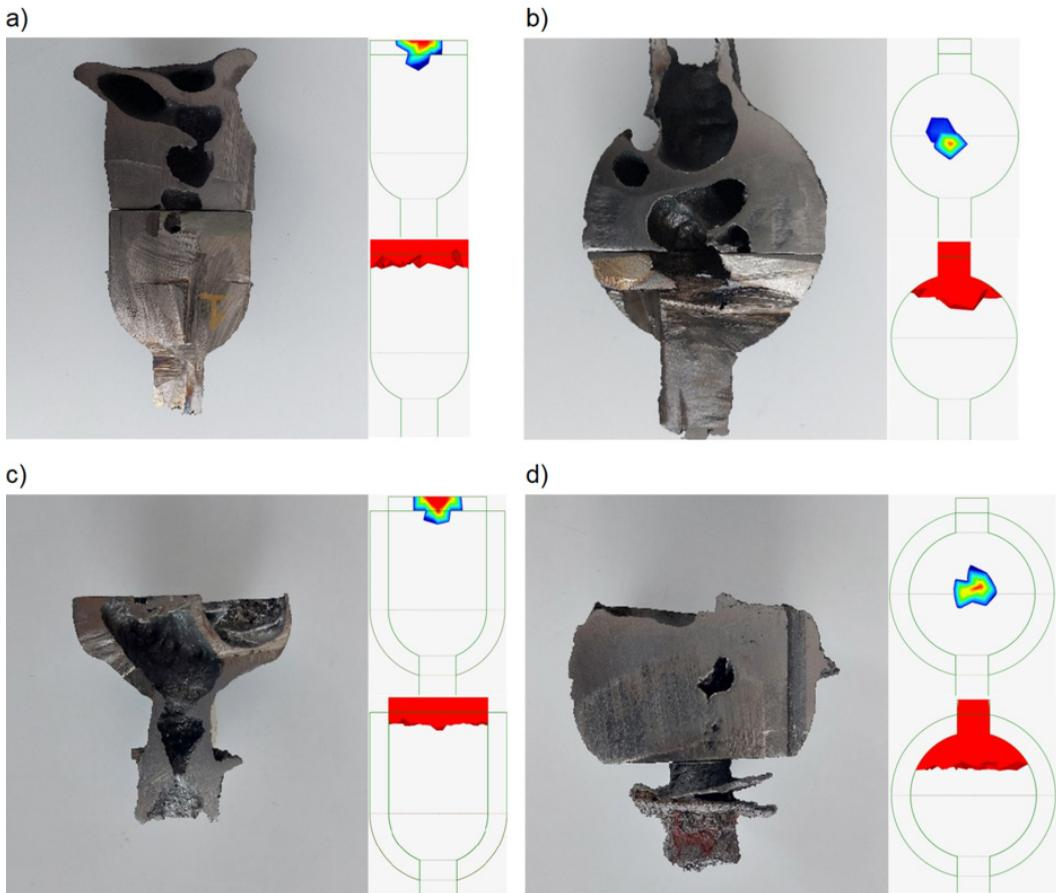
observed that for an initial volume of 100%, the exothermic riser sleeve with a cylindrical shape is the one with better area exhibits. However, when the volume is reduced, the exothermic riser sleeve with a spherical shape is the one with a better area.
