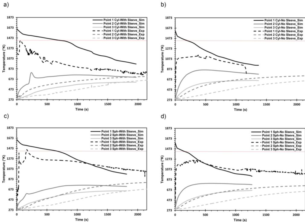
to the values of 60% size conventional risers. This clearly shows that the use of exothermic sleeves improves the behavior of the riser.
