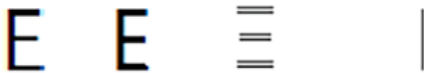
Original Image Smooth Sub-image (SS) Horizontal Sub-image (OS) Vertical Sub-image (SO) (c) Wavelet decomposition of the character "E"
