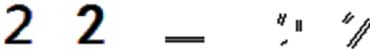
Original Image Smooth Sub-image (SS) Horizontal Sub-image (OS) Vertical Sub-image (SO) Diagonal Sub-image (OO) (a) Wavelet decomposition of the digit "2" at a single scale
