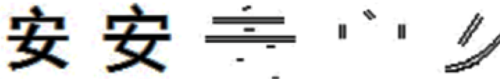
Original Image Smooth Sub-image (SS) Horizontal Sub-image (OS) Vertical Sub-image (SO) Diagonal Sub-image (OO) (b) Wavelet decomposition of the Chinese character "安" (An)
