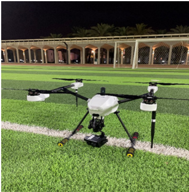
Figure 2. A quadrotor drone equipped with a color/infrared (IR) camera for data collection
