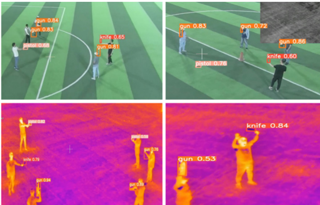
Figure 6. Small “you only look once” version 5 (YOLOv5s) prediction results for color video (top) and infrared video (bottom)
