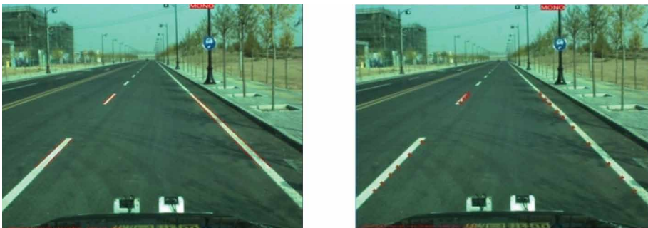
Figure 6. Left: Candidates of lane boundary lines. Right: Selected boundary points.
