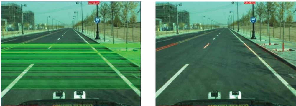
Figure 4. Left: A set of scan lines. Right: Examples of detected edge points; input image is as shown on the left.
