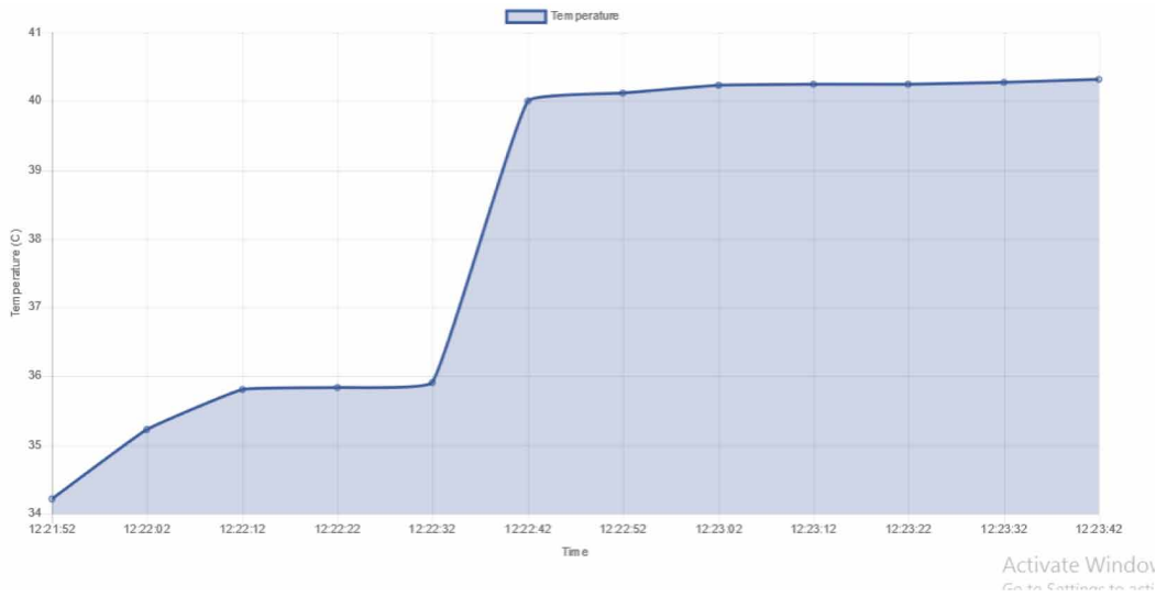
Figure 9. Temperature chart from combustion of inflammable liquid
