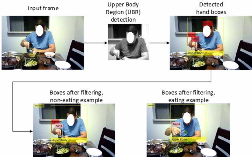
Figure 14. Samples of the eating process detection and tracking showing successful eating event detection for persons who is dining
