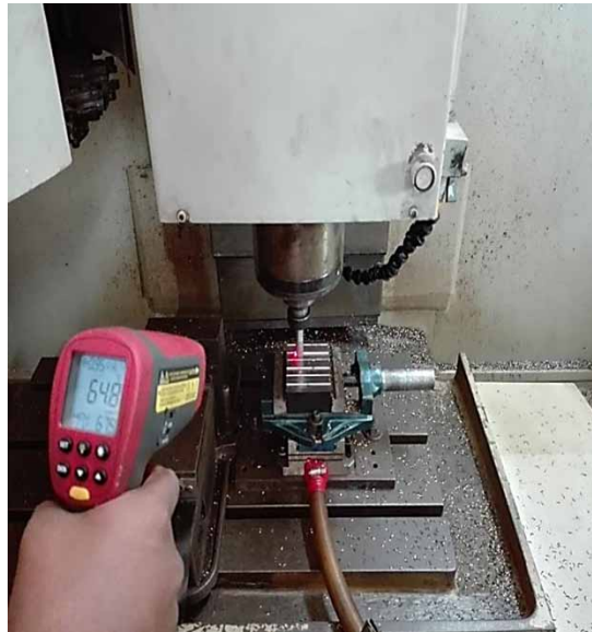
Figure 2. Measurement of cutting temperature
