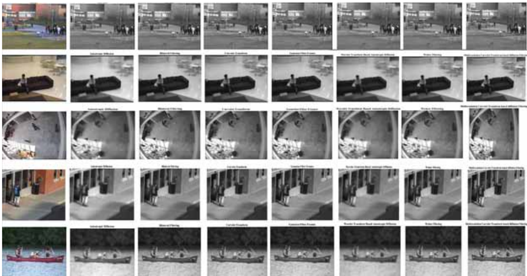
Figure 5. Snapshots taken from the five scenes where column 1 represents the original frames, column 2 represent the anisotropic diffusion based denoising and column 3 represents the bilateral filter based denoising, column 4 represents the curvelet denoising, column 5 represents the gaussian denoising with median filtering, column 6 represents wavelet based anisotropic diffusion based denoising of the foreground, column 7 represents the weiner denoising process and column 8 represents the proposed curvelet based denoising where row 1 represents the crowd in university, row 2 represents person sitting on a sofa, row 3 represents 2 people fighting, row 4 represents the person waiting on the bus station and row5 represents a moving canoe
